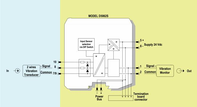
Input configuration selection via internal Dip-Switch
