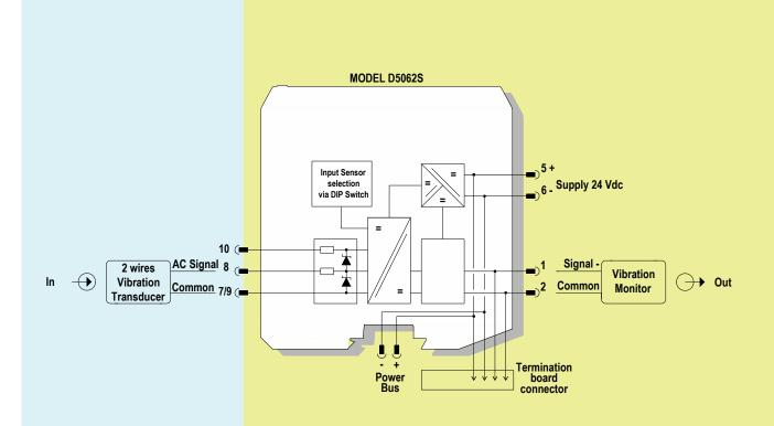
Input configuration selection via internal Dip-Switch
