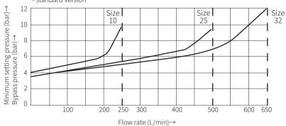
Minimum setting pressure and bypass pressure in relation to the flow - "U" version
