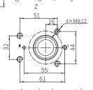
It must be ordered separately if connection subplate is needed. G51/01 (G1/4"); G51/02 (M14x1.5)
