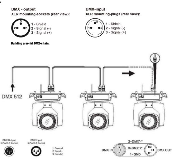
Connect the DMX-output of the first fixture in the DMX-chain with the DMX-input of the next fixture. Always connect one output with the input of the next
