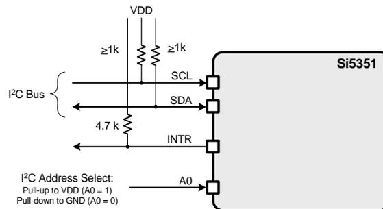
**Figure 7. I<sup>2</sup>C and Control Signals**
