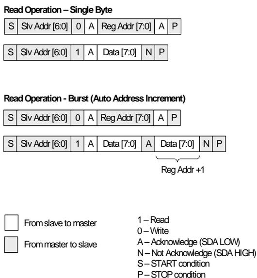
**Figure 10. I<sup>2</sup>C Read Operation**
