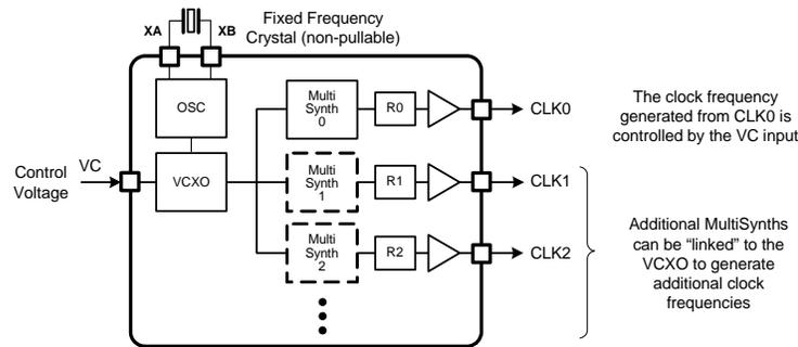
Figure 5. Using the Si5351 as a Multi-Output VCXO
