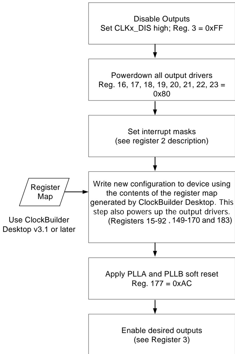
**Figure 12. I<sup>2</sup>C Programming Procedure**
