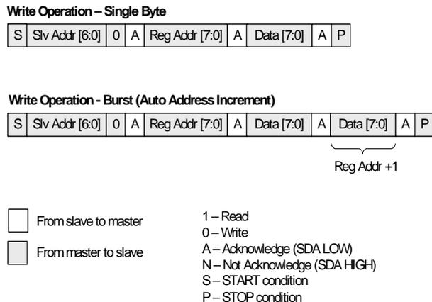
**Figure 9. I<sup>2</sup>C Write Operation**
