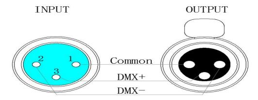
**CAUTION:** Do not allow contact between the common and the fixture's chassis ground. Grounding the common can cause a ground loop, and your fixture may perform erratically. Test cables with an ohm meter to verify correct polarity and to make sure the pins are not grounded or shorted to the shield or each other.
