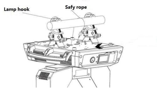
Mount the fixture using a suitable "C" or "O" type clamps. The clamps should be rated to hold at least 10x the fixture's weight to ensure structural stability. Do not mount to surfaces of unknown strength, and ensure properly rated rigging is used when mounting fixtures overhead.
