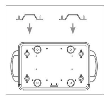
Attach the 2x 1/4-turn quick lock Omega brackets to the base, and the clamps to the brackets.
