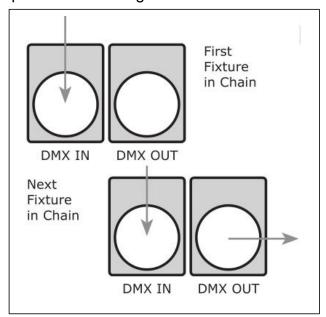
A quick note: Often, the setup for Master-Slave and Standalone operation requires that the first fixture in the chain be initialized for this purpose via either settings in the control panel or DIP-switches. Secondarily ,the fixtures that follow may also require a slave setting.
