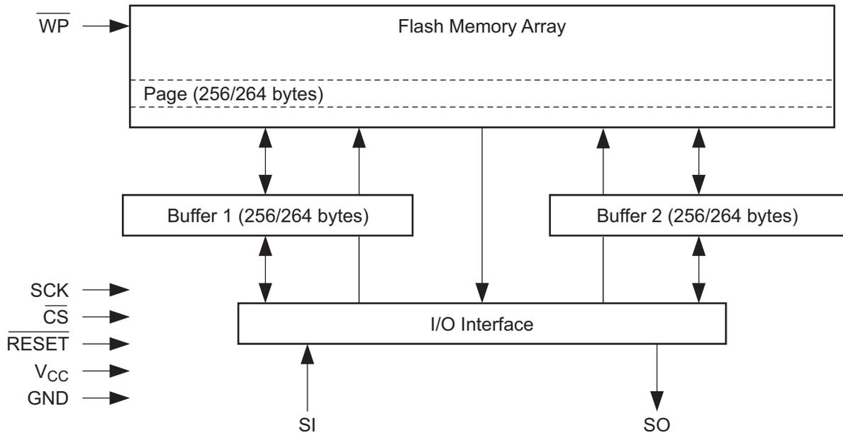
Figure 23-2. Buffer Write
