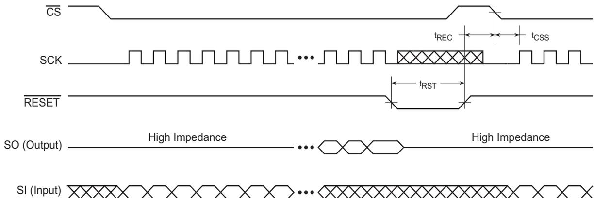
Note: 1. The  $\overline{CS}$  signal should be in the high state before the  $\overline{RESET}$  signal is deasserted.
