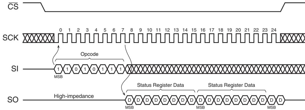
**Figure 25-11. Manufacturer and Device Read (Opcode 9Fh)**
