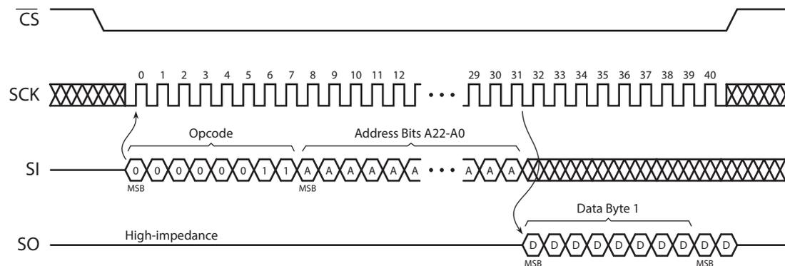
Figure 25-7. Read Sector Protection Register (Opcode 32h)
