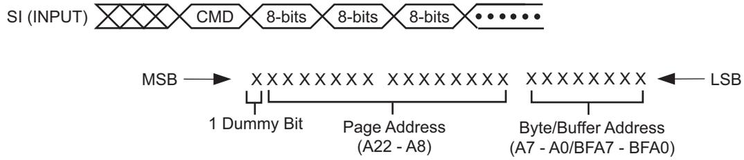
**Figure 21-3. Command Sequence for Read/Write Operations for Page Size 264 bytes**
