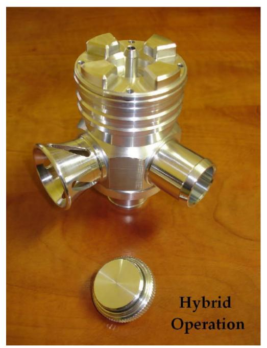
If the user chooses to setup the valve in a **100% recirculating configuration**, the discharge horn will need to be removed (unscrewed) and replaced with the blanking plug on the body of the valve. Nothing else will need to be change for this particular configuration of the valve. Please see below:
