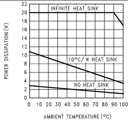
Figure 17. Maximum Power Dissipation (TO-220)
