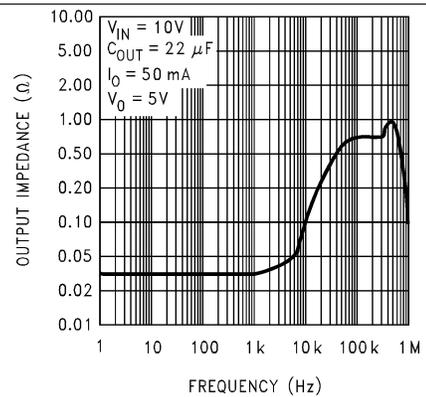
Figure 10. Output Impedance
