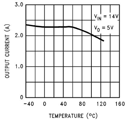
Figure 16. Peak Output Current
