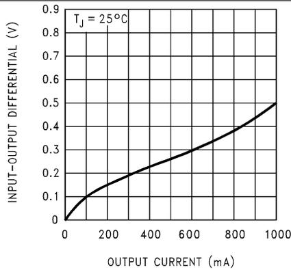
Figure 1. Dropout Voltage
