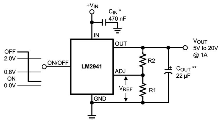
$$V_{OUT} = \text{Reference voltage} \times \frac{R1 + R2}{R1} \text{ where } V_{REF} = 1.275 \text{ typical}$$
