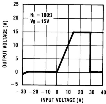
Figure 15. Output at Voltage Extremes
