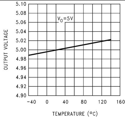
Figure 3. Output Voltage
