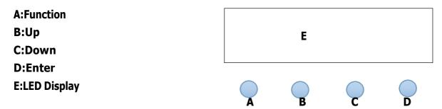
Instructions:Press the function key A cycled out the eight different function effects, digital tube first two digits on behalf of which the current function(see menu). The last two digits represent the functions in which the address code or speed parameters. Press the B or C key to modify the parameter values. Press the D key to confirm.
