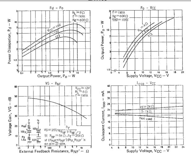
Output power (reference value) corresponding to supply voltage and load resistance.
