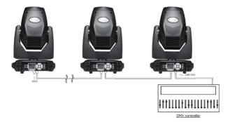
Connect the DMX-output of the first fixture in the DMX-chain with the DMX-input of the next fixture. Always connect one output with the input of the next fixture until all fixtures are connected.
